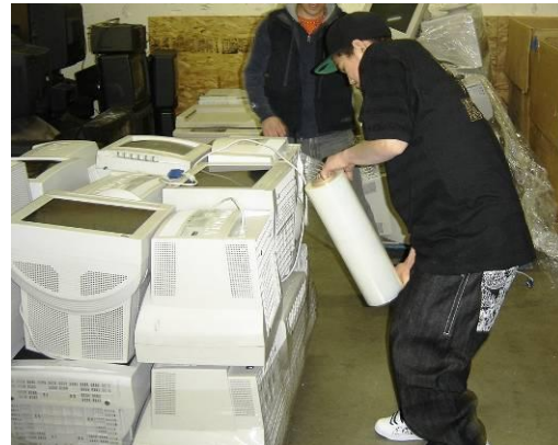
Once the monitors are two rows high, the stack can be wrapped
