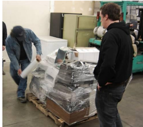
Finishing off a pallet by tightly securing it with stretchwrap
